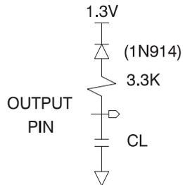
Note:  $CL = 100 \text{ pF}$  including jig capacitance except -55 devices, where  $CL = 30 \text{ pF}$ .
